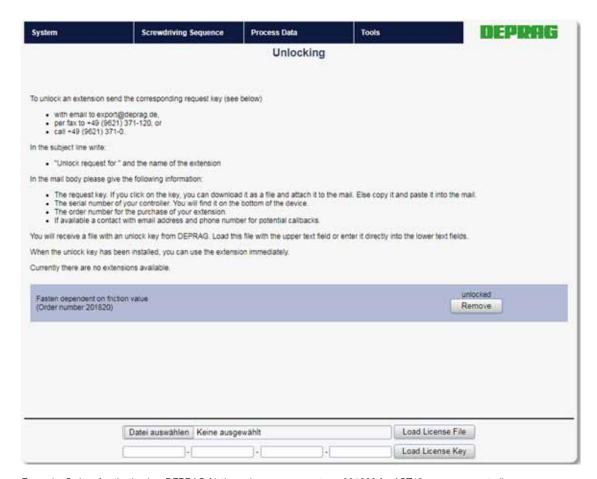
Example: Order of activation key DEPRAG friction value process, part no. 201820 for AST40 sequence controller
