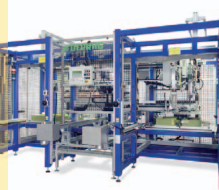
Screw assembly of a radiator grille
